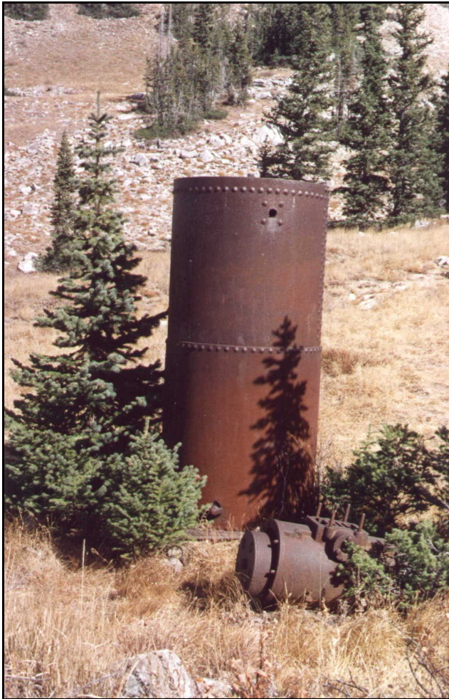
Fig. 1. The boiler that provided steam for the fifteen-horsepower engine that drove a pump to move water from the adjacent springs to the Prince of Wales mine nearly a mile away still remains on the flat a short distance below the Twin Lakes Pass. Parts of the pumping machinery while away the years with the boiler.
