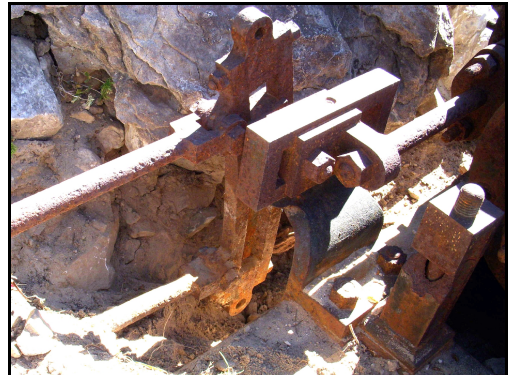
Fig. 5. This photo shows the link with the two eccentric rods coming in from the left. The valve rod runs off to the right to the steam valve. Notice the vertical slot in the link, allowing it to be moved up or down by linkage from the Johnson Bar, not seen here due to its being buried in the debris. When the engine is running the link continuously rocks back and forth, its vertical position determining the amount of motion transmitted to the valve rod.
