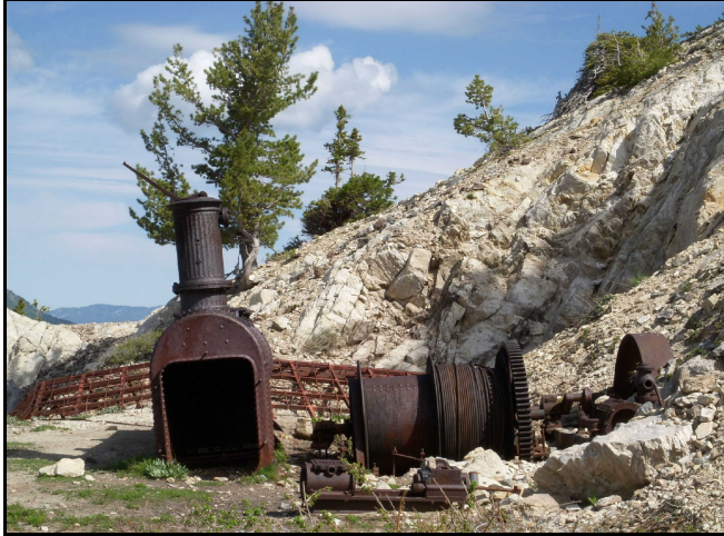
Fig. 1. The boiler at the Prince of Wales mine generated steam for the thirty-horsepower engine and hoist that lifted ore and other material out of the shaft and lowered men and material. The hoisting machinery is to the right of the boiler. The shaft is covered by a metal grate seen in the background.
