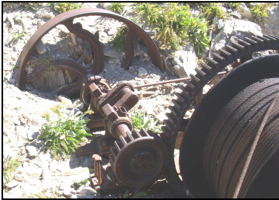
Fig. 4. This photo shows the crankshaft with the flywheel at the far end and the cable drum in the foreground. The cams, cam followers and one of the eccentric rods can be seen between the flywheel and crankshaft throw.
