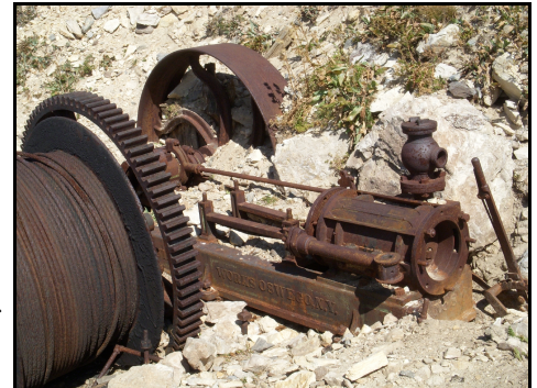
Fig. 2. Overall view of the steam engine and hoisting drum. The Johnson bar control and disassembled cylinder are at the right, flywheel in the background and cable drum in the foreground.
