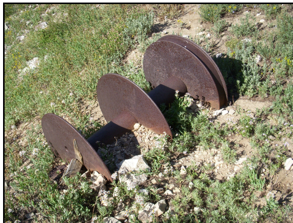
Fig. 2. A large metal spool remains on the dump at the Davenport tunnel, a remnant of the tramway that ran down to Grizzly Flat.
