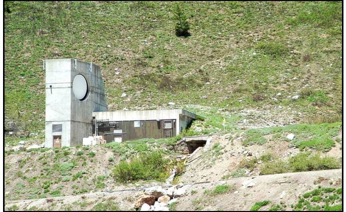
Fig. 1. The culvert at the right side of the telephone building north of the Peruvian Lodge in Alta marks the site of the Howland tunnel. The portal was on the other side, and in its day the tunnel’s snowshed ran through the culvert. The Little Cottonwood highway runs across the bottom of the photo.
