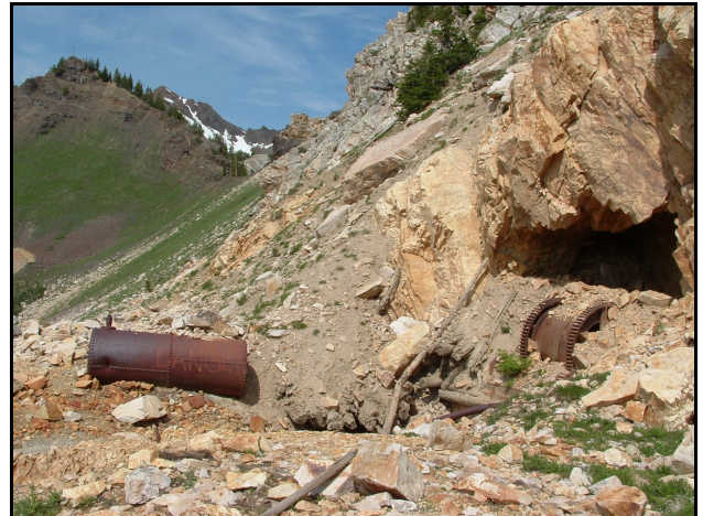
Fig. 4. The huge hoisting engine, idle for more than a century, still rests in its cave-like shelter behind the Toledo shaft, almost buried by dirt and rock that has come down over the cliff. The shaft is covered with a metal grate, which also has collected its share of rocks. The tank on the left was an air tank, an accumulator to store compressed air from the compressor house in the canyon bottom. The air was used to drive the hoist and the water pumps down inside the mine.
