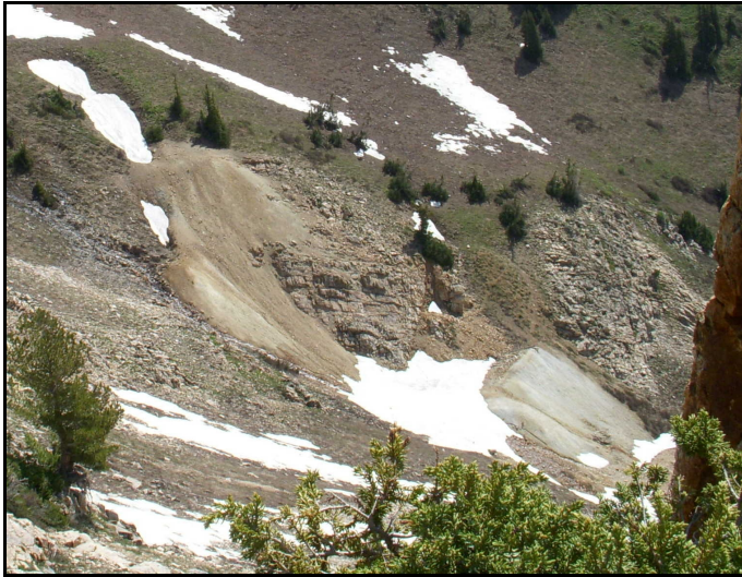
Fig. 3. Springtime view of the Emily mine as seen from the cliffs to the southwest. The depression created by the collapsed incline shaft at the top of the dump is filled with snow, as is the collapsed No. 1 tunnel at the upper left side of the dump. The Henderson tunnel is completely covered by the snowbank over the lower dump.
