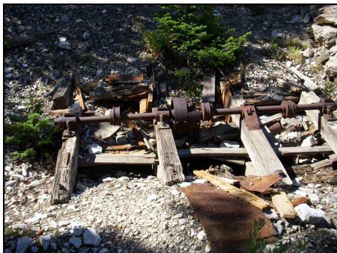
Fig. 4. Remains of a shaker table used to concentrate ore remnants remaining in the dump below the Number Four tunnel.
