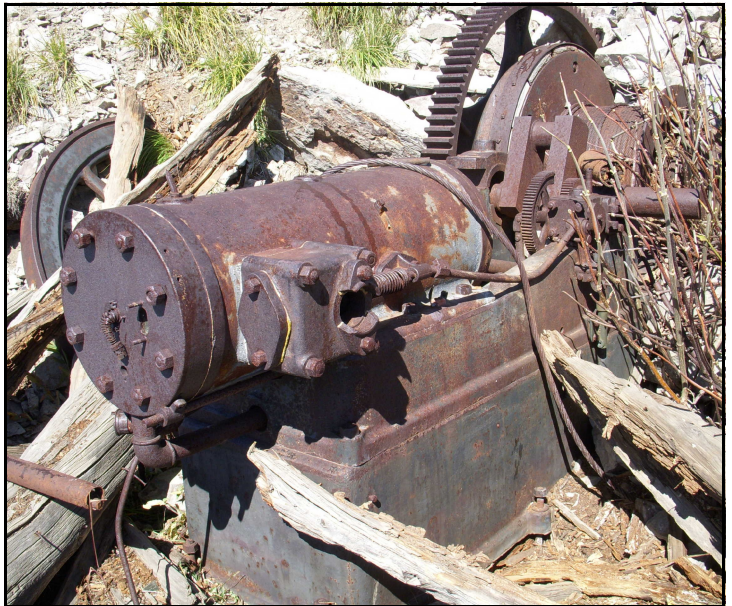
Fig. 4. The Fairbanks-Morse hoisting engine was installed at the mine in 1902. It is a sadly damaged, rusted and partially dismantled example of the classic 'hit and miss' type of engine popular in the early twentieth century. The large flywheel, an essential component of this type of engine, has been removed and is seen under the debris in the background.
