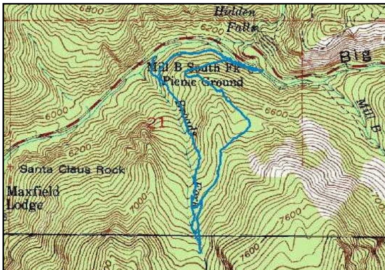
Fig. 2. In addition to the trail and road shown in Figure 1, this figure shows the logging slide running down to Big Cottonwood creek and the flume right of way for the Big Cottonwood Power Company's proposed "Borck Fork" (Broads Fork) power plant.
